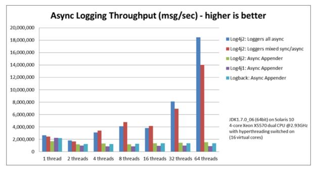
On Solaris 10 (64bit) with JDK1.7.0\_06, 4-core Xeon X5570 dual CPU @2.93Ghz with hyperthreading switched on (16 virtual cores):
