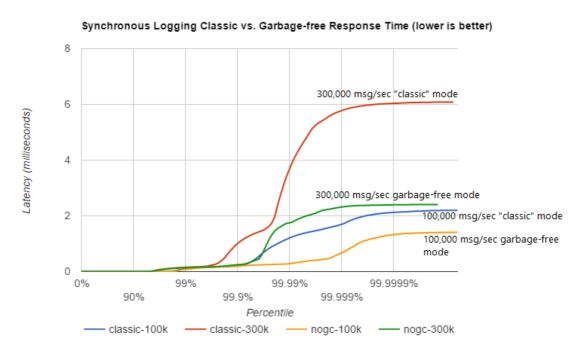
The above results are obtained with the ResponseTimeTest class which can be found in the Log4j 2 unit test source directory, running on JDK 1.8.0\_45 on RHEL 6.5 (Linux 2.6.32-573.1.1.el6.x86\_64) with 10-core Xeon CPU E5-2660 v3 @2.60GHz with hyperthreading switched on (20 virtual cores).
