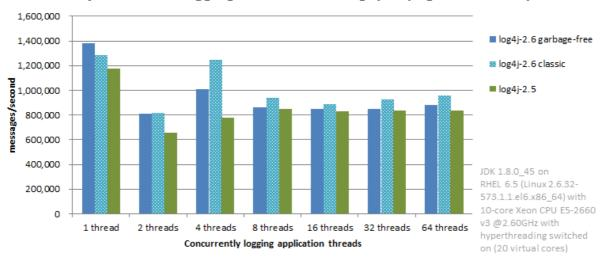
The results above are obtained with the JMH Java benchmark harness. See the FileAppenderBenchmark source code in the log4j-perf module.
