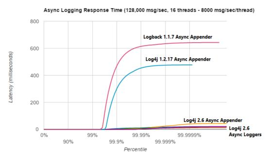
The graph below zooms in on the Log4j 2 results for the same test. We see that the worst-case response time is highest for the ArrayBlockingQueue-based Async Appender. Garbage-free async loggers have the best response time behaviour.
