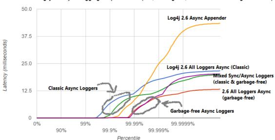
Log4j 2.6 Async Logging Response Time (128,000 msg/sec, 16 threads - 8000 msg/sec/thread)
