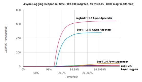
The graph below zooms in on the Log4j 2 results for the same test. We see that the worst-case response time is highest for the ArrayBlockingQueue-based Async Appender. Garbage-free async loggers have the best response time behaviour.
