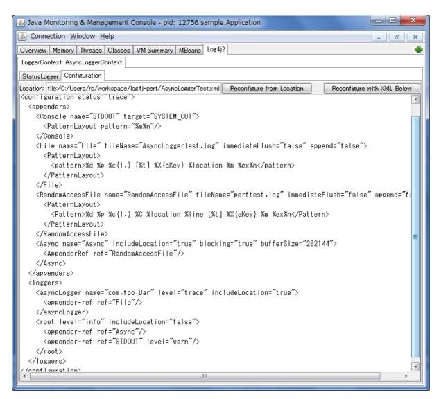
The configuration edit panel provides two ways to modify the Log4j configuration: specifying a different configuration location URI, or modifying the configuration XML directly in the editor panel.
