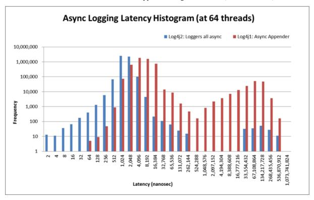
Note that this is log-scale, not linear. The above graph compares the latency distributions of an asynchronous logger and a Log4j 1.2.17 Async Appender. This shows the latency of one thread during a test where 64 threads are logging in parallel. The test was run once for the async logger and once for the async appender.
