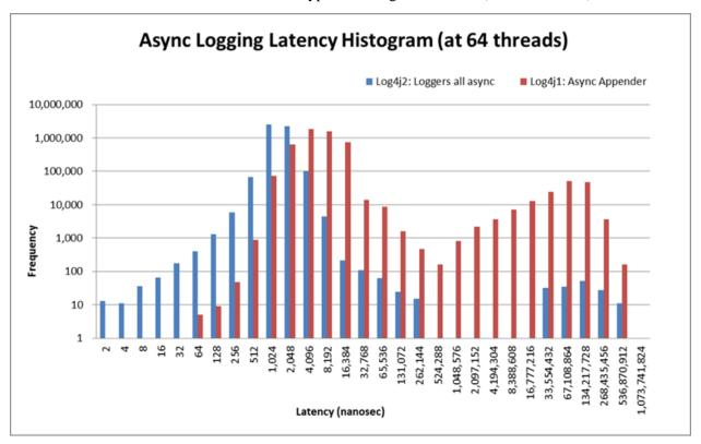
Note that this is log-scale, not linear. The above graph compares the latency distributions of an asynchronous logger and a Log4j 1.2.17 Async Appender. This shows the latency of one thread during a
