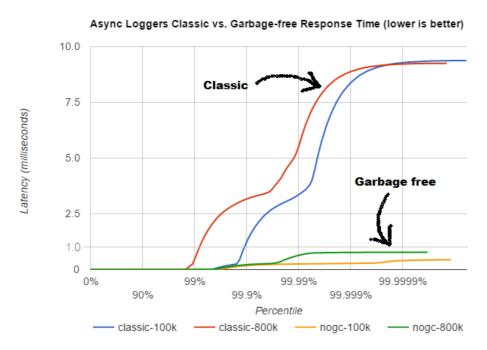
In **classic** mode we see numerous minor garbage collections which pause the application threads for 3 milliseconds or more. This quickly adds up to response time delays of almost 10 milliseconds. As you can see in the graph, increasing the load shifts the curve to the left (there are more spikes). This makes sense: logging more means more pressure on the garbage collector resulting in more minor GC
