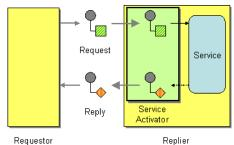
Components like Bean, CXF and Pojo provide a a way to bind the message exchange to a Java interface/service where the route defines the endpoints and wires it up to the bean.
