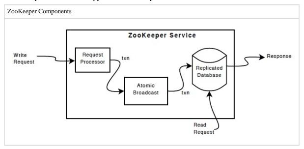
The replicated database is an in-memory database containing the entire data tree. Updates are logged to disk for recoverability, and writes are serialized to disk before they are applied to the in-memory database.
