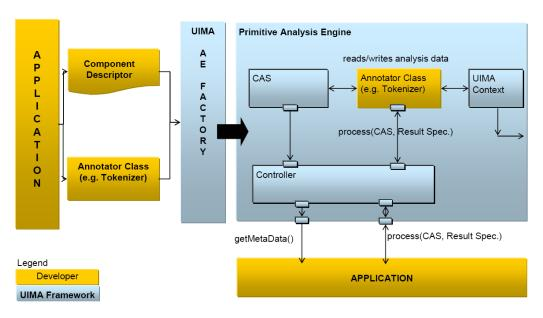
Figure 2.4. Using UIMA Framework to create and interact with an Analysis Engine
