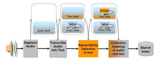
Figure 2.7. Multiple Sofas in support of multi-modal analysis of an audio Stream. Some engines work on the audio "view", some on the text "view" and some on both.
