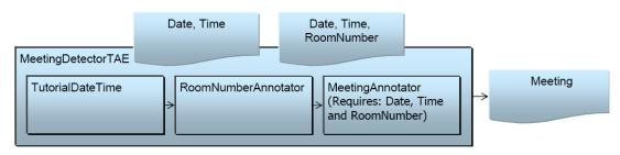
Figure 1.2. An Aggregate Analysis Engine where an internal component uses output from previous engines
