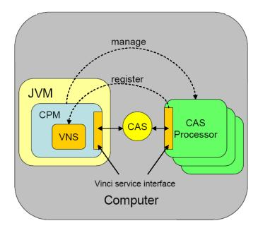
Figure 2.3. CPE with Managed CAS Processors
