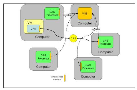
Figure 2.4. CPE with non-managed CAS Processors
