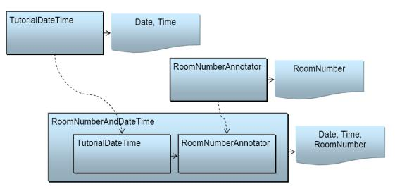
Figure 1.1. Combining Annotators to form an Aggregate Analysis Engine
