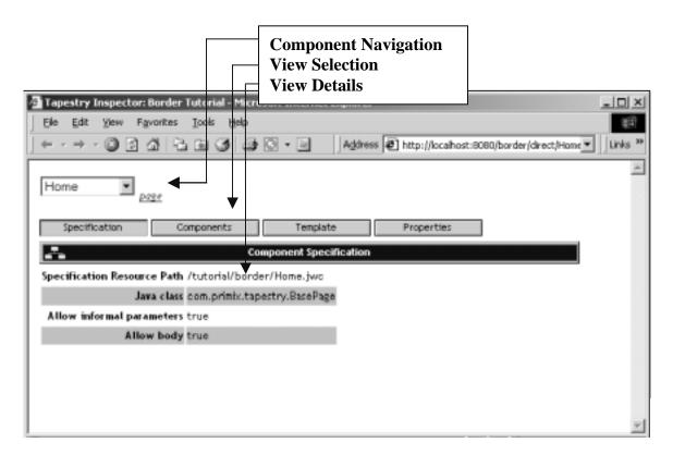
The Inspector displays live information from the running application; in fact, it is simply another part of the application (the drop-down list of pages will include the Inspector page itself). The Inspector is most often used to debug HTML generation by viewing the HTML templates.
