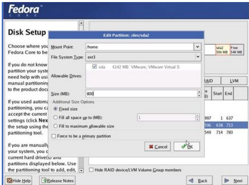
Illustration 11: Repeat the above step for other mount point. Linux requires the minimal to be / (root), and swap
