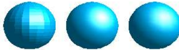
Figure 10 - Shading examples. From left to right: Flat, Phong, Gouraud.
