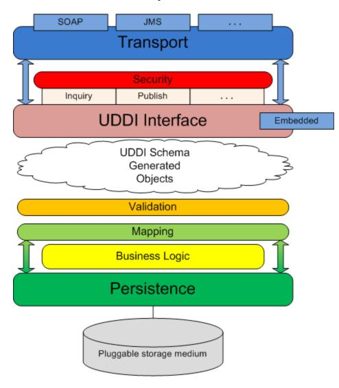
The diagram above shows the software layers and components employed in the jUDDI project implementation for UDDI v3. Here is a brief description of each item in the diagram and how they all work together to create the UDDI-compliant registry that is jUDDI:
